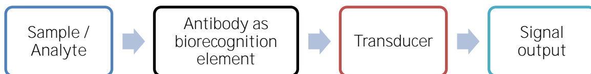
Figure 4.5 - General principle of an immunosensor.
