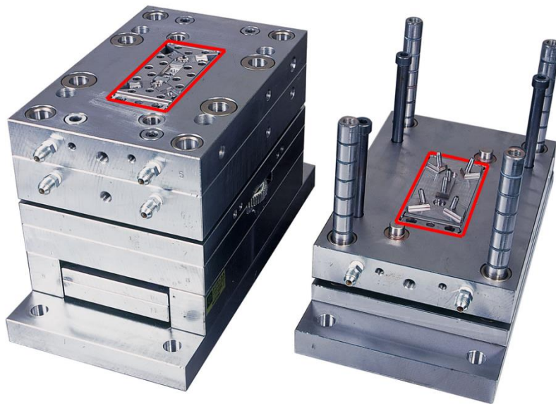
Figure 6.15 – The entire mould where the inserts are marked with a solid red line ( http://tsquality.ch/- )
