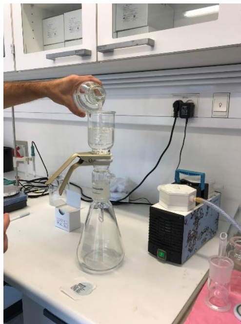
Fig. A.1 The water sample collected from the tanks were filtered using 0.45 \mu\text{m} pore sized 47mm dia sterilized filter papers from Advantec. The setup is as shown in figure. All the glassware were washed thoroughly with ultra-pure water and ethanol.
